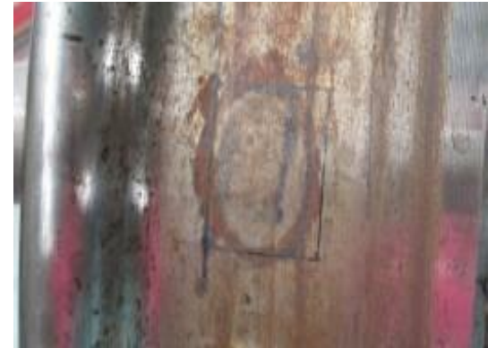
Circumference defects of wheel rim
