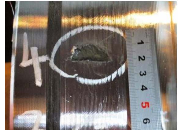
Crack with 10mm length and 30mm width, 10mm below the wheel rim tread
