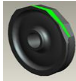
AP probe: Radial defect detection in wheel flange
