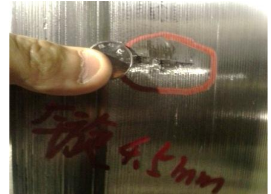
Crack with 5mm length and 30mm width, 8mm below the wheel rim tread
